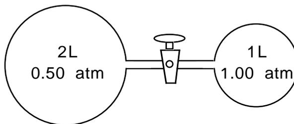
Hydrogen gas is contained in two vessels connected by a closed stopcock as shown in the diagram. The volumes and pressures are also shown. When the stopcock is opened and the gases allowed to mix at constant temperature, the final pressure will be (neglecting the volume of the tube between the bulbs)
